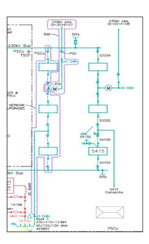
Figure 1 – Preliminary one-line of GI-2016-7 POI within the Boone 230kV Substation
